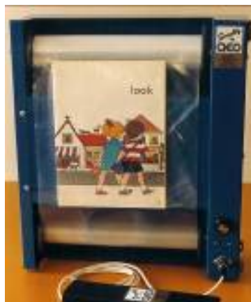
The Possum typewriter equipment, showing the electronic control surmounted by an enlarged code unit
